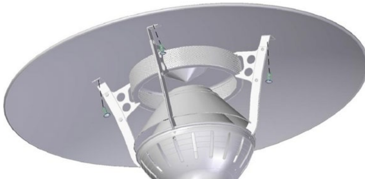
Figure 7: Attach Top Reflector to Shield Support Arms
