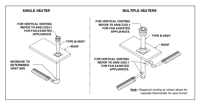
Note: Horizontally vented heaters must be individually vented and cannot use a common vent.
